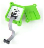
Figure 3. Keolabs IoTize module Source: Keolabs
